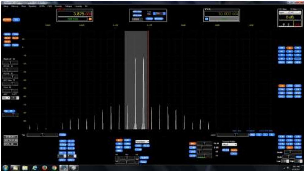
To the left is the Two Tone Test with “Pure Signal Engaged” Below left is the same Two Tone Test but without “Pure Signal Engaged”
